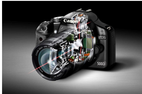
Görsel 8.1. DSLR Fotoğraf Makinesi Kesiti (creative-photographer.com)
